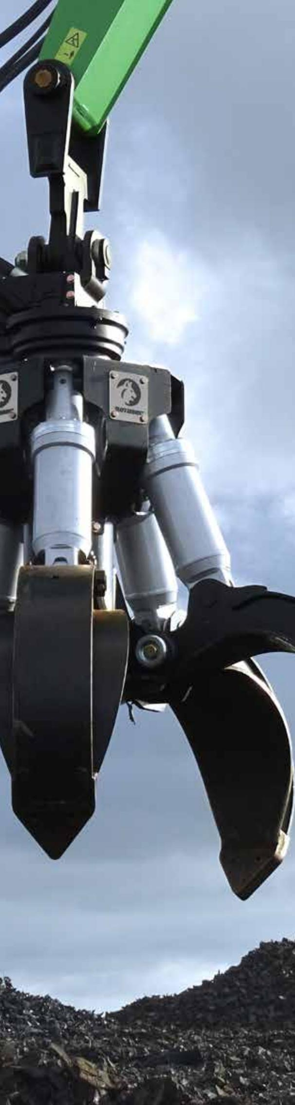
A large, detailed view of an orange peel grapple attachment on a green excavator arm. The grapple has two large, curved tines and is positioned over a pile of dark material. The background is a cloudy sky.
